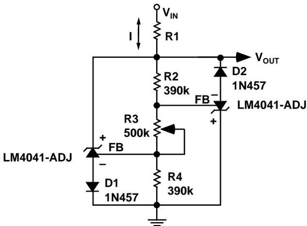
Figure 7. Bidirectional Adjustable Clamp
