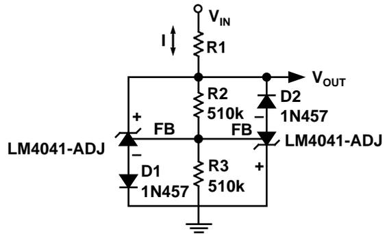
Figure 6. Bidirectional Clamp
