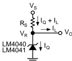
**Figure 1. LM4040, LM4041 Fixed Shunt Regulator Application**
