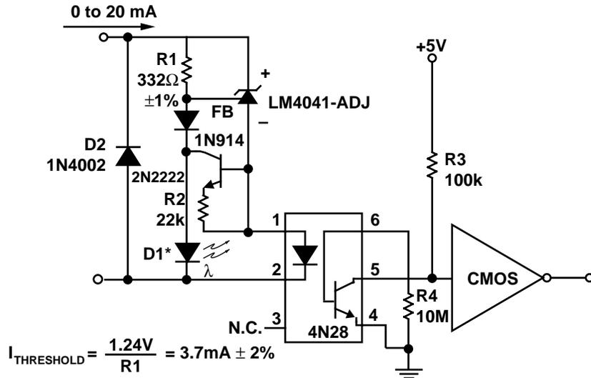
\* D1 can be any LED,  $V_F = 1.5\text{V}$  to  $2.2\text{V}$  at  $3\text{mA}$ . D1 may act as an indicator. D1 will be on if  $I_{\text{THRESHOLD}}$  falls below the threshold current, except with  $I = 0$ .
