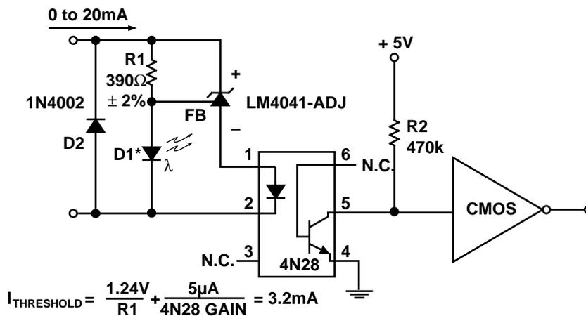
\* D1 can be any LED,  $V_F = 1.5V$  to  $2.2V$  at  $3mA$ . D1 may act as an indicator. D1 will be on if  $I_{THRESHOLD}$  falls below the threshold current, except with  $I = 0$ .
