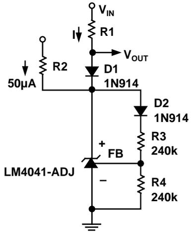
Figure 5. Fast Positive Clamp
