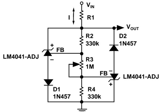
Figure 8. Bidirectional Adjustable Clamp
